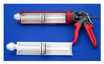
This picture illustrates a full universal cartridge. The plunger/rod of the caulking gun is fully extended.
